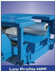
Ideal for low discharge height machines and offers better filtration than traditional flat bed paper filters
