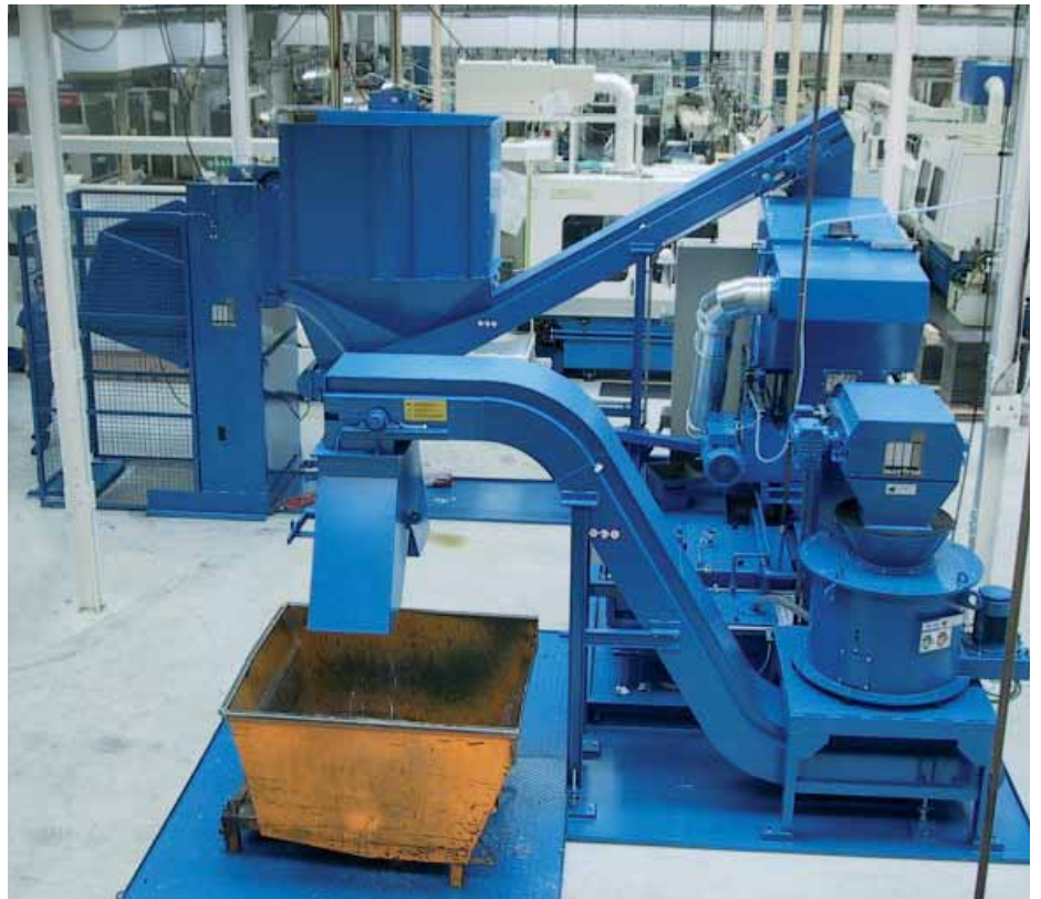
Installation consisting out of following components: chip-wringer, chip crusher, chip-conveyor and container loading system.
