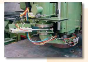
Tailor made extraction hoods, having a 360 degree annular design, complete with auto opening for tool changing, wear resistant quick release skirts, coolant spray nozzles and quick release removal flanges.
