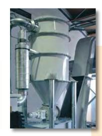
Low volume, high pressure extraction systems would have high pressure extraction fan set or side channel blower depending on design characteristics. The product and air are separated in a filter cyclone with the initial coarse particle separation taking place in the main chamber and the secondary air is passed through a filter cartridge and product is deposited via the rotary valve located at the base of the unit.
