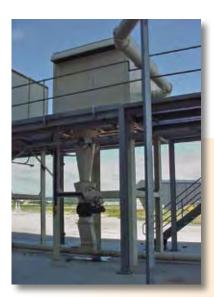
Air separation cyclone unit having a heavy duty mild steel construction complete with removable wear liners to suit applications.
