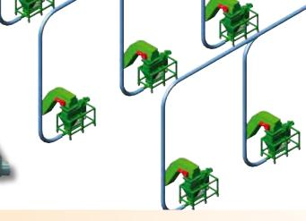
Purpose made collection hopper complete with cross flow silencer, auto shut off and sequencing dampers, level sensing, support frame with heavy duty castors and quick release "Cup and Ball" type connection. Unit can be disconnected and pulled clear in case of breakdown or maintenance.
