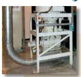
Rotary Airlock to allow product input without air leakage. Supplied with flexible blade tips to cope with the risk of tramp parts. Heavy cast iron version
