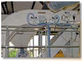
Product feed chutes that are suitable for multiple conveyors. Available with pneumatic diverters, sound dampening liners and bin fill level sensing devices.
