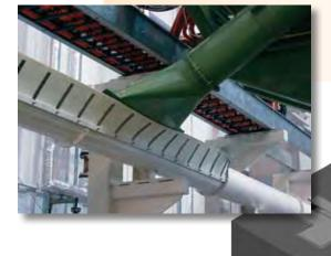
Custom telescopic sections to allow for vertical Z axis travel complete with linear actuator, precision bearing slideways, gauge length measurement and close tolerance ptfe/nylon air seals.
