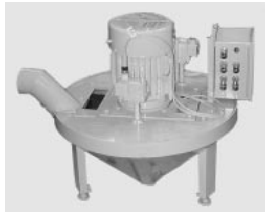
Tank with pump—no conveyor
