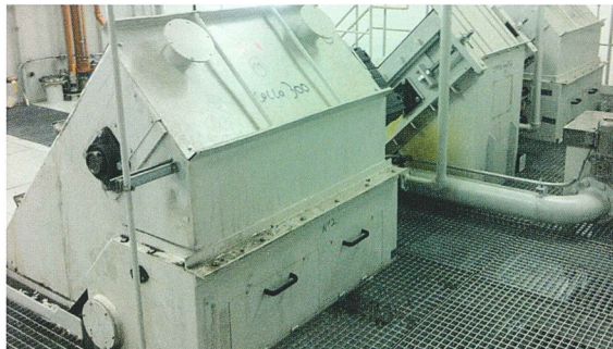
Discharge End of a VacuFilter E-Series Central Coolant System, supplied to a steering component manufacturer
